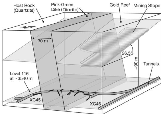
**Figure 1.** Sketch of the location of the JAGUARS network in the Mponeng gold mine and its surrounding geologic formations. The JAGUARS network is located at 3540 m depth. The sensors are located in boreholes that are shown as bold black lines. The PG dike is shown in gray. The gold reef with active mining located above the JAGUARS network is shown in light gray. The mining stope width is 0.5–1 m. The development tunnels XC45 and XC46 are shown in dark gray.
